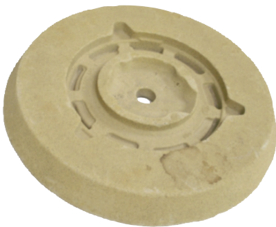
A steel mould made from Delf sand by a foundry
